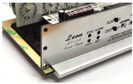
Next remove the buttom cover from the enclosure and add the electronics plus a reinforcment profile as shown in the photo.
