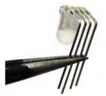
7.: Pick up the RGB-LEDs and bend them as shown in the picture. Keep special care about the location of the Anode wire (longest wire)
