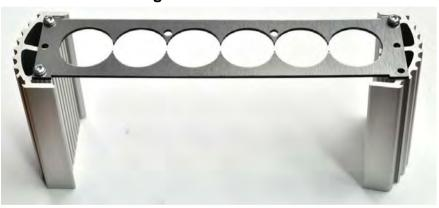
Pick up the front cover, remove both protective films and att ach the cover on the aluminium profiles. Now fix the cover only with 3 screws GF M3 x 14 and tighten loose the right hand screw.
