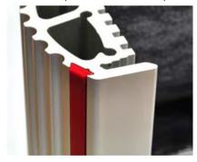
Add four rods to the aluminium profiles. Keep care about the correct orientation of the nut.
