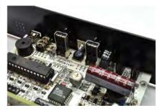
Remove from the rear cover the protective film from the self-adhesive side (the engraved outer side has no film) and fix it on the main board with the M3 x 6 screw
