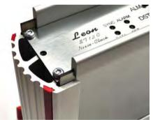
Slide carefully the electronics together with the buttom cover into the enclosure. Check if the neons will fit into their holes on front. Next fix the rear with the remaining 4 x GF M3 x 14 screws
