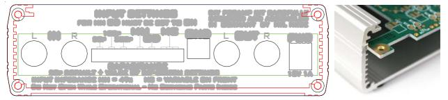
Next fit on the bottom of the aluminium profile the four black adhesive feet to the corners of the large flat surface. Now slide the mainboard into the second groove from above as shown in the picture.
